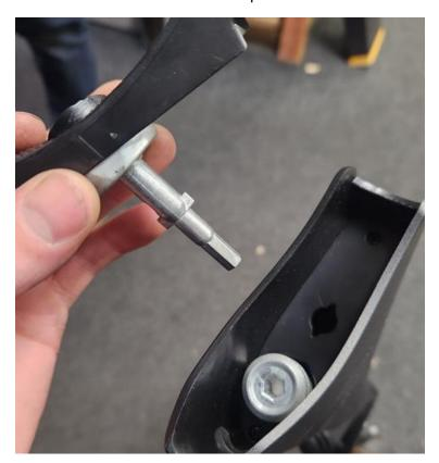
3: Using the stock cover, unscrew the stock screw. **Caution: Avoid unscrewing the stock screw if the gas pressure is still high in the rifle.**
